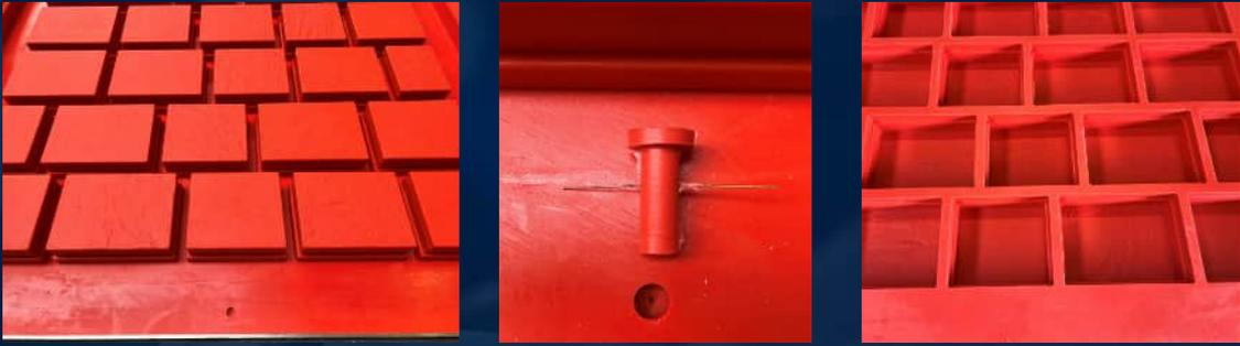
The slide features three red-tinted images illustrating the assembly process. The first image shows a grid of rectangular blocks labeled 'Modell'. The second image shows a red cylindrical component labeled 'RFID Tag' being inserted into a hole in a red surface. The third image shows a grid of rectangular blocks labeled 'Wetcast Form'.
